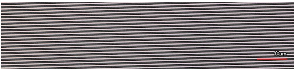
Stitching free large areas of single frequency gratings
