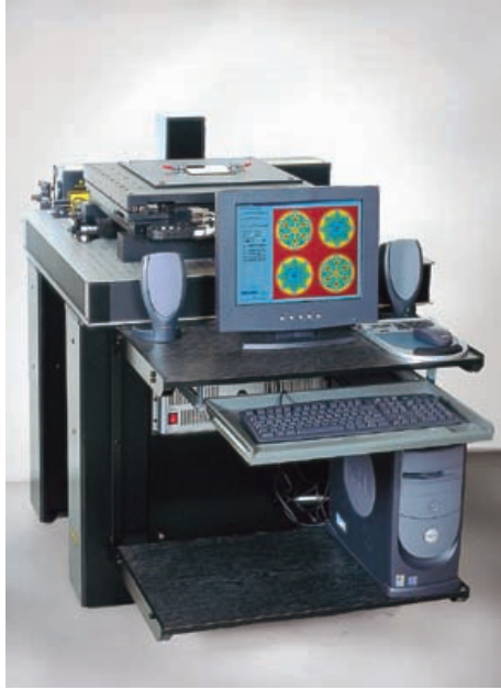
The Lightgate System 1270, 1997, utilising a Helium Cadmium laser.
